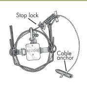
Figure EC32. Powered cable device (set)
