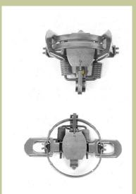
Figure EC13. wide jaw, offset trap
