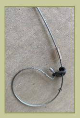
**Figure BC26.** Reichart 180-degree bend washer lock
