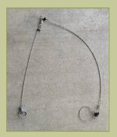
**Figure BC25.** Non-Powered Cable Device with Reichart 180-degree bend washer lock
