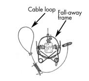
Figure BC21a. Powered cable device
