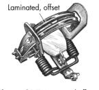
Figure OP7. Laminated offset trap
